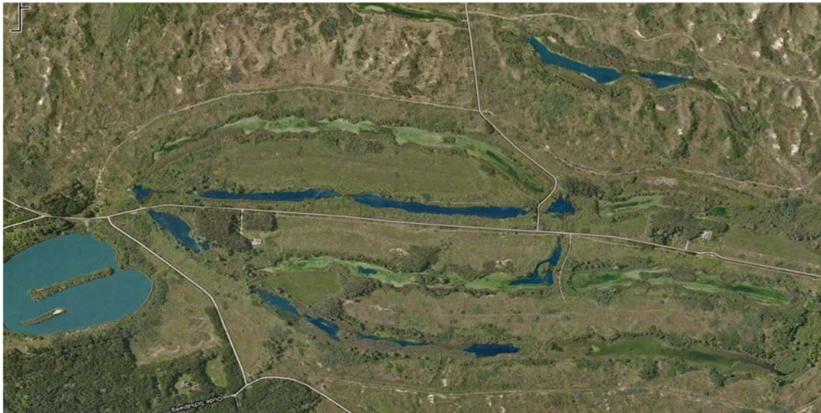
Fig. 1, Aerial View of Castricum Dune Infiltration Area. Surface water, after some pretreatment, is fed into canals. Water is abstracted from a long row of wells between two canals (shown in red dashed lines)
